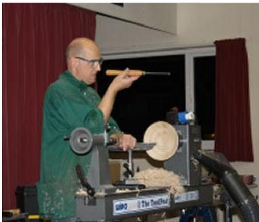
A technique new to me, but probably old-hat to most of you was demonstrated during the hollowing of the bowl. As a means of getting a better finish in the bottom of the bowl the tool handle was dropped and the attack angle changed as the gouge was swept up and round and down to the centre as Mark explained taking best advantage of the speed of the lathe to produce a better finish on the last couple or so centimetres. (I have since tried this and so far it works for me)
