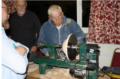
when rough turning a blank about 10mm bigger than gripping size (when the jaws allow for truing up the finish turn the piece.
