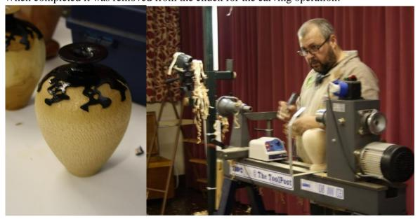
As you can see from the picture (I'm not sure whether it was Mick's hands shaking or mine) the tool used was a dentists' style drill, but electric, fed from a variable speed control box and the cutters were very small, very short tungsten carbide milling blades. The cutting was done freehand taking care to ensure the rotation of the cutter was with the grain direction to reduce the chance of
