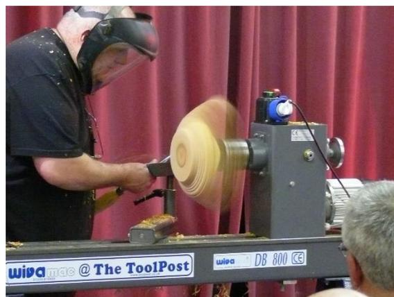
The centre of the bowl was finished with a shallow ground conventional bowl gouge and after sanding would be finished with a matt oil. Shaun believes the beauty is in the wood not in what's added afterwards
