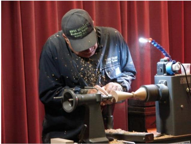
The picture shows the bottom of the piece being finished after being parted off and mounted on a jam-chuck
