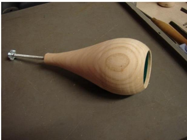
After shaping showing key-nut rod.
