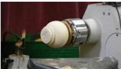
Using a compression chuck made from a scrap piece of wood and cut to fit the threads, the head was reversed in the chuck and sanded to a finish. The eye and ear positions were marked out and drilled for fixing (under normal conditions the head would have been hollowed out). The Eyes were made from ebony dowels and were glued in position cut and sanded to finish.
