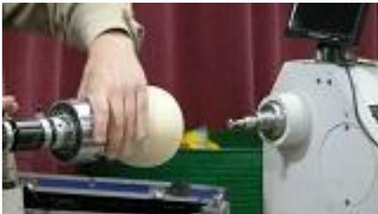
The chuck with body attached was removed complete to ensure that the alignment was maintained. The thread turning jig was fitted into the tail stock and the centre height checked to matching the headstock. A 16 tpi thread cutting head was mounted in the headstock. The jig being preset at 16 tpi was indexed forward until there was a slight 'kiss' between the wood and the cutting head.
