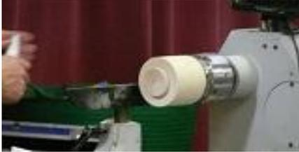
The head section was then turned until it was proportionate to the body (rule of thirds apply). Cutting the neck section to be 1mm greater than the body aperture was checked by the callipers to ensure sufficient material to create the thread.
