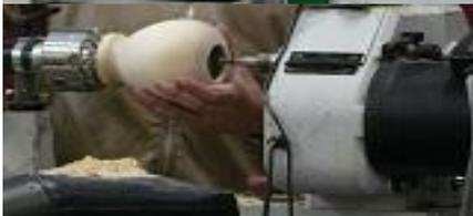
The 16 tpi thread required indexing a further five positions on the jig coming out clear between each index and repeating until the neck of the body had a clean thread cut. (Again it is worthwhile to watch the video).
