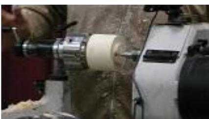
Again to ensure correct alignment Simon removed the chuck and head complete before screwing onto the jig assembly. This time it was easier to see the thread being cut because it was on the outside edge. Super glue was again used before and during cutting to harden the wood and give a cleaner cut, using an activator spray to ensure it was dry before cutting. (Its worth looking at the video on this as well, as a picture can paint a thousand words, and certainly does it better than I can).
