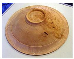
A waste piece was mounted on the lathe and given a curved surface. Some tissue was placed over it and the face of the bowl held in place with the tail stock and the base finished.
