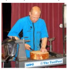
After mounting it between centres he proceeded to true up the edge then the face using pull cuts with a swept back gouge as well as creating a spigot for reverse mounting to complete the face of the platter.
