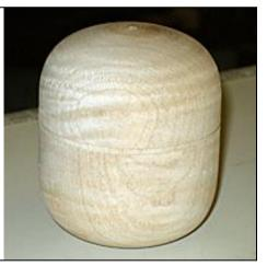
After mounting, rounding off and creating spigots at either end, he parted off a section for the lid. He made a recessed lip and began hollowing. Once again he starting with the ring tool and used it in combination with a scraper to complete the hollowing process.
