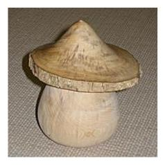
The other piece was then mounted and the end grain face was finished off with a central recess. This was to be the lid and the base was offered up and checked for fit, adjusting the recess as necessary.
