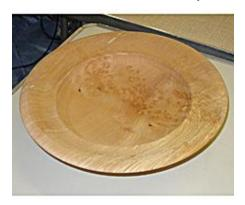
Moving towards the centre of the platter, he created an undercut rim for the middle bowl whilst explaining his choice and use of gouges in order to get the required finish.
