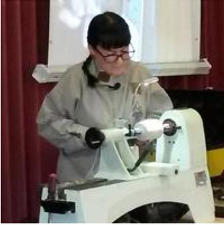
She then proceeded to turn a spigot on one end and mounted the piece in a chuck. It was now ready for drilling out the inner sections to accommodate the lower part of the pepper mill mechanism.
