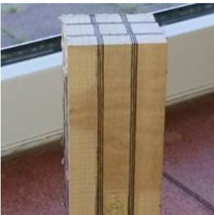
The base of the pepper mill was Maple and had two laminated sections on each of the four sides. It was mounted between centres and turned to round at which point she double-checked that it was truly centred on both ends by reducing them using a parting tool and checking that the laminations appeared equal on all sides. This is crucial to ensure the finished design is correct.
