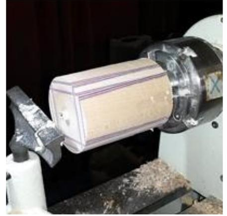
This did not go all the way through as she needed to leave some depth of wood for the top end where a recess will be needed for the upper part of the mechanism.
