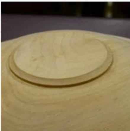
The first 12in piece was mounted on a screw chuck and the tail stock brought up for added support and safety. It was trued up on both faces using the larger bowl gouges. A 1mm deep spigot was then turned on the foot. A very small amount to grip on usually, but Mick explained that with his new Record SC4 Chuck and large jaws set at the optimal diameter (i.e. an exact circle) there would be a 360deg grip and would therefore be sufficiently safe. Something to consider for all turning projects.
