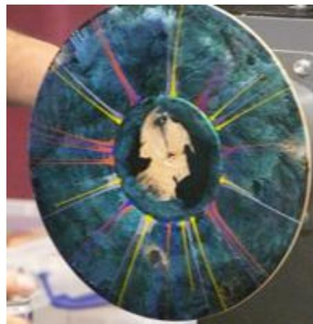
Blobs of colour were then applied around the central rim where the bowl section was to be. The lathe was turned on and a plastic cover held over the piece to prevent paint flying everywhere. The result was radiating lines of colour towards the outer edge. A second colour was applied, turned and dried. This allowed for a colour to be overlaid on the previous ones without them blending together. The net result was lacquered to finish.
