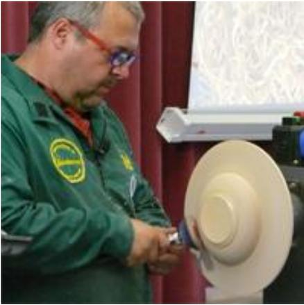
A 3in sanding arbor with 320 grit paper was used on the base followed by a combination of 20% bees wax and 80% oil to seal the surface.
