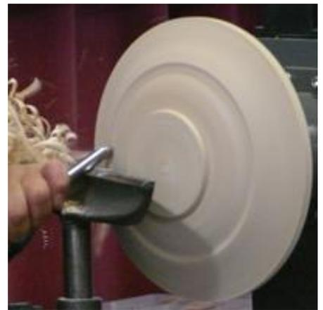
Mick then turned away the underside allowing for a bowl in its centre and a wide rim to the outside edge. As he worked he removed wood in a step-by-step process and emphasised the need for good posture and position when turning as well as sharp tools. Finishing with a push cut using his 1/4 bowl gouge.
