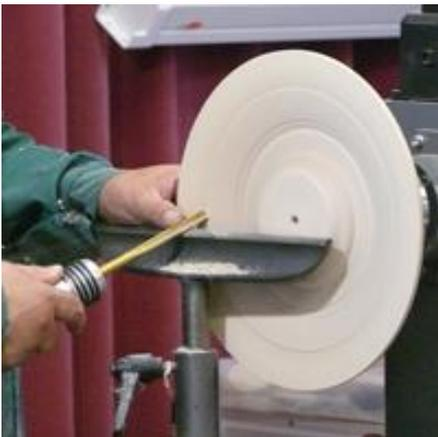
The large bowl was mounted on the SC4 Record Chuck and proceeded to true-up the face and shape the outer profile only. The centre core was left till last in order to stabilise the timber.
