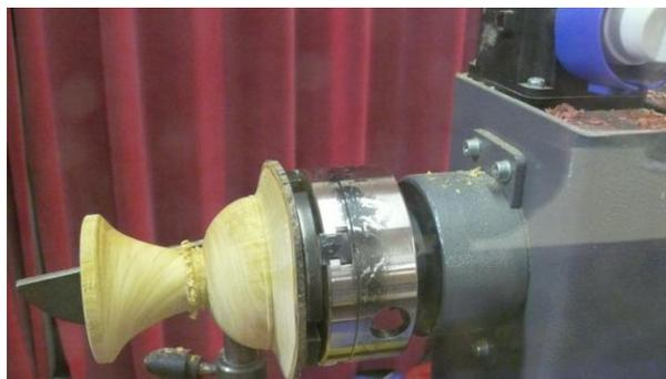
Using the base as a jam chuck adjustments were made until the lid fitted satisfactorily bearing in mind that the wood was not kiln dried and likely to move.
