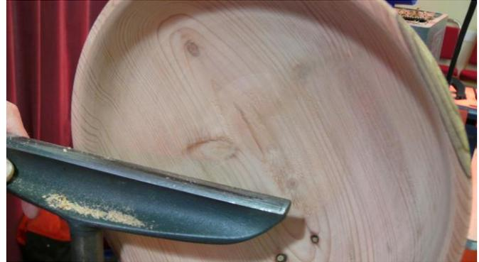
Having a 2nd bevel (heel) helps to drive the tool round curves whilst refining the shape. Under normal circumstances the piece would now be sanded through to 600 grit but a pad would be necessary as finger pressure may cause peaks and troughs.
