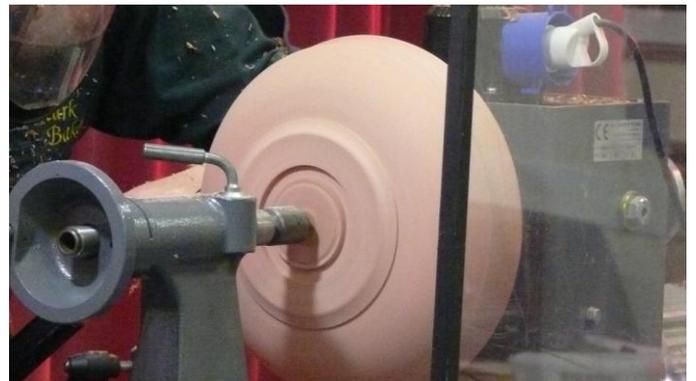
Mounted between centres Mark used a pull cut to true up the face, and because of the imbalance he also trimmed the opposite side, again using a pull cut.
