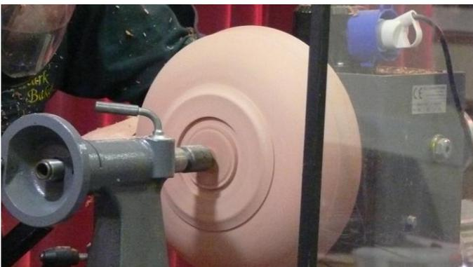
Mark proceeded to form the OG shape using a push cut with a 10mm bowl gouge, because of the harder areas within the wood he wished to avoid excessive sanding with coarse grits as this would cause peaks and troughs, however using a square scraper a good finish can be obtained. (A shear scrape was attempted which resulted in grain tear out).
