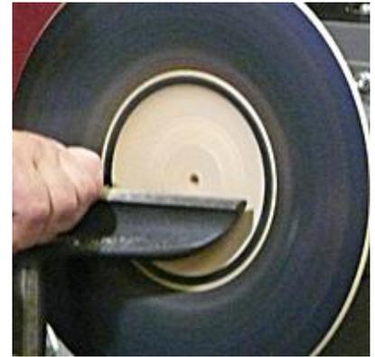
Whilst this piece was being passed round the 8" blank was turned in a similar way but Mick created a slightly different shape, again ensuring the spigot was the correct size for the chuck so that it was gripped equally all round the edge. The wax/oil mix was again applied during sanding from 240 through to 400 grit. This process really emphasized the ripple grain pattern within this piece of sycamore.
