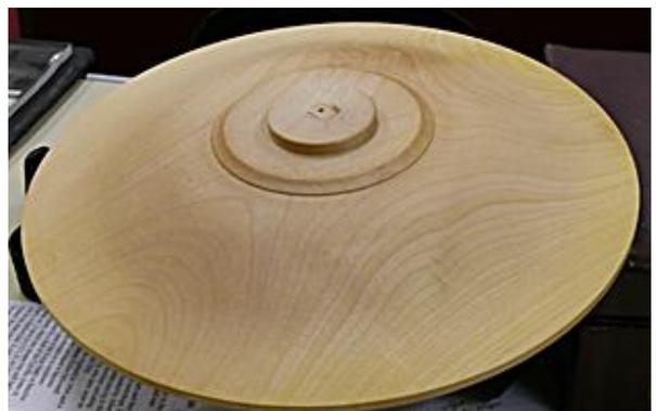
Using a 15mm bowl gouge with a shallow 60 degree grind the face and edge were cleaned up and the underside of the platter formed. A compression spigot and a foot approximately one third of the diameter of the platter were formed and the final finishing cut was made using a quarter inch bowl gouge. Whilst creating the ogee shape from the foot using a shear cut Mick emphasised the need for sharp tools if you are to achieve the required finish.
