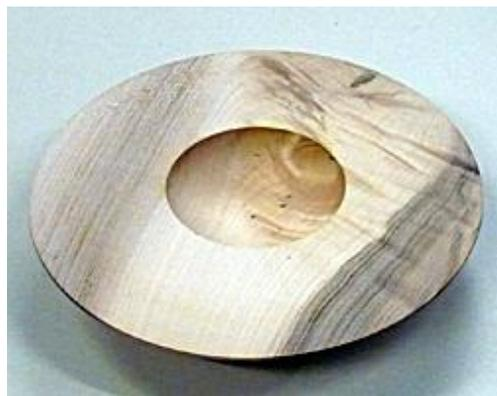
It is always good practice to sharpen the tool before a final cut, the correct passage and shape of the tool will avoid bevel rub bruising and using the correct arc will ensure a pimple, if anything, is left which is easier to remove than a dimple. Finally the centre was sanded again using oil/wax mix to 400 grit.
