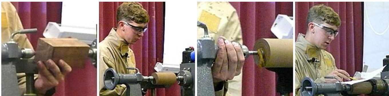
Ryan then produced the piece of Ebano (a very dense wood) which was mounted between centres and turned to round with a Roughing Gouge once again using a parallel tool rest. A tenon was added to one end to fit the lathes chuck jaws. It was turned and mounted in the jaws. A Skew was used to square off the base end before a Jacobs Chuck was put into the tail stock and a 20mm Forstner Bit used to drill a 43mm deep hole.
