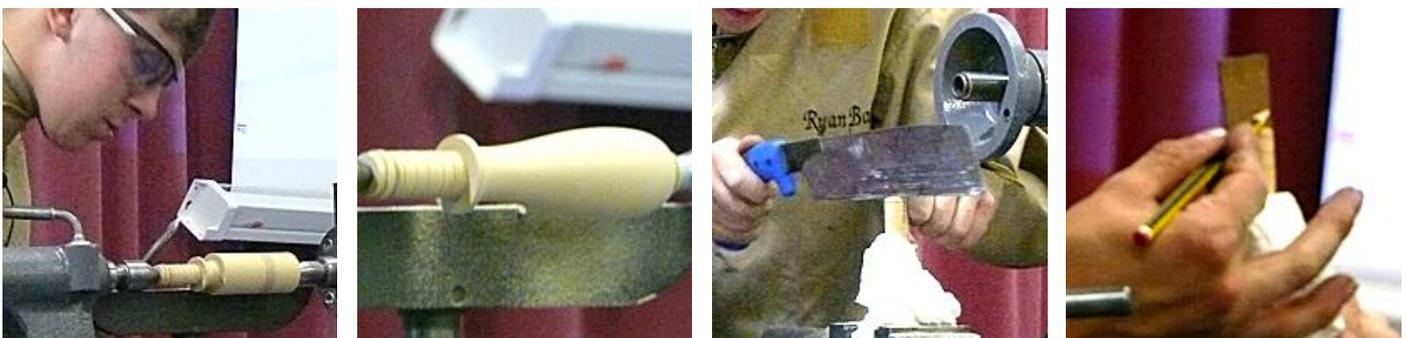
The handle was then put into temporary jaws so that Ryan could cut a small "V" down the middle of the tenon using a pull saw, into which a thin wedge would be placed. A small wedge was then pushed gently into the "V" and marked at 3mm above the end. This was done because the mortice on the head piece would be drilled to 40mm deep and the fillet on the handle accounted for another 3mm.
