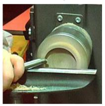
The top section was then mounted on the lathe. The depth of the protruding tenon on the base was checked and the same amount was hollowed out of the lid. The face was squared off to ensure an accurate, gap-free join with the base. After a great deal of fine adjustments the base and lid came together to create the finished turned "square" box. As a way of finishing off the box Andy turned a bead on the lid and formed a shallow recess in the middle.
