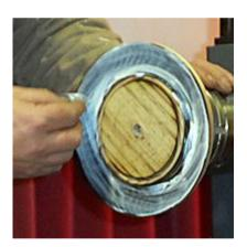
The surface of the scorching was removed by light sanding leaving a light and dark ribbed effect due to the Ash's natural growth rings. Liming wax was then applied and normally allowed to dry for about a day. However, Andy didn't have the time and so proceeded to remove the excess wax creating the finished effect as best he could. The outer edge was cut and rounded off, then the middle hollowed out thus creating a lovely deep bowl with a delightful contrasting rim.
