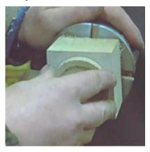
At the bottom of the recess was a raised outer ring, with the middle being 1-2mm deeper. After checking that the inner faces were flat and square, he applied CA glue. The tenon insert was sprayed with accelerator and forced home using the tail stock and a block of wood as a clamp.
