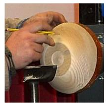
Andy prefers to create a tenon on the base of bowls as a compression fit is a much safer way of holding the piece as opposed to a recess where the expanding chuck jaws could apply too much internal pressure and split the bowl causing a potential safety hazard. Andy was using a Crown Bowl Gouge made of M42 steel, which he knows gives a superior and longer lasting cutting edge. The outside was then shear-scraped, leaving only a small amount of sanding to get a good finish.
