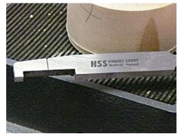
The next hole was drilled, again pre-marked using a 40mm bit and the crush grind tool used to shape the recess. The body was then mounted and a 25mm hole was drilled right through.
