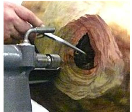
During this getting started part of the demonstration Darren had to work hard to remove wood on a slow turning heavy piece as a lot of the time he was "cutting" fresh air. He used a 5/8in bowl gouge for this.
