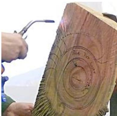
The outer sections at each end were to have a textured finish. To create this he used a 50mm Proxxon circular carver with a chain saw cutting disc. As he did this he was careful to score the lines as if they were radiating from the middle of the piece.
