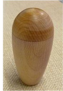
The base was then hollowed out with a spindle gouge by using it initially to create a hole in the middle then shear scraping outwards. A bowl gouge and scraper were used to finish the inside and bottom. The feathery waste was cleared away and plastic mesh placed over the piece and held in place using tape. The mesh is often used as a protection over sharp tools and metalwork. Simon Hope uses it on his hollowing tools.
