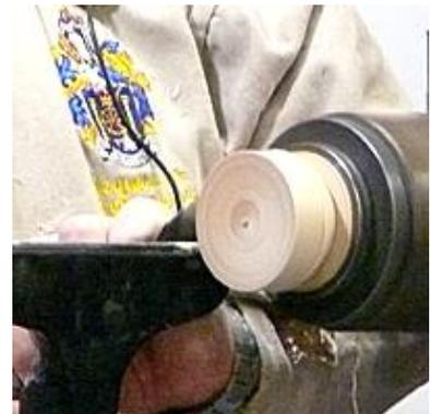
The other piece was then mounted in the jaws and a slightly tapered spigot created with the skew, the lid was offered up and the spigot adjusted until the lid fitted perfectly. The tail stock was brought up and the waste wood turned away.
