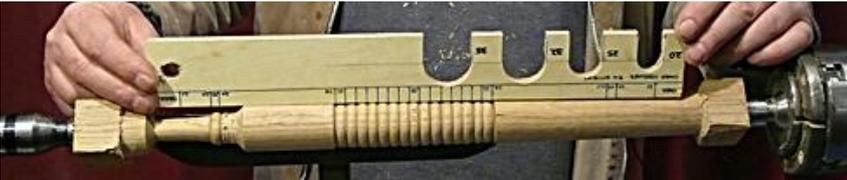
The divides between the beads were marked using the skew and Andy then used his 1/4in beading tool to roll the beads into shape. He recognised that many people use a specially shaped beading tool for this purpose but that they were effectively scrapers and would not necessarily produce the same quality finish as the flat edge of a beading tool.
