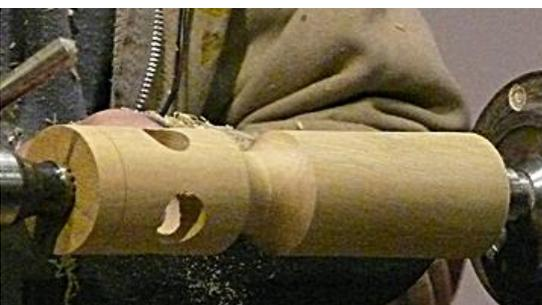
To add a little interest to the piece three small v-cuts were made and a black feature ring created by using a small piece of Formica to burn the line into the wood.
