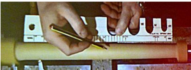
A Witness Stick comprises a length of 3/8<sup>th</sup> ply with the positions of all the spindle elements marked along one edge. On the opposite edge various sized cut-outs were created that were to be used as gauges for the different size spindle sections in order to recreate the same diameter sizes as the original.
