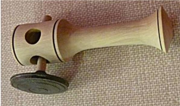
The top was put into one of the holes of the launcher and a small hole drilled centrally. A suitable thread was put through the hole and the top turned to wind it on. The thread is then pulled and the spinning top launched on to the chosen surface.
