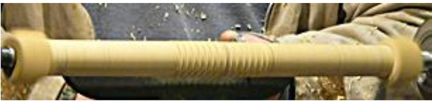
The shaping of the spindle was mostly with a skew chisel to ensure minimal sanding. In doing so he discussed the benefits of mastering the skew, one of which was creating the beads in the middle section of the spindle.
