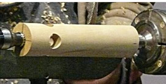
It was mounted between centres and turned to a cylinder. A cove was firstly cut 20mm below the holes using a spindle gouge, where Andy discussed how important it was to cut down across the grain in order to get a good clean finish as opposed to cutting upwards and tearing wood the fibres. The cove was then extended towards the base of the piece to create the handle section. The top and bottom ends were marked and turned down using a parting tool.
