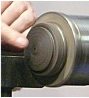
For the spinning top Andy suggested that any scrap pieces of wood could be used. First up was to produce the stem of the top. A 1in square spindle was mounted and turned to approximately 1/3<sup>rd</sup> the size of the holes in the launcher. It was sanded smooth and parted off at a length about 30mm longer than the diameter of the launcher.
