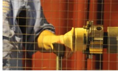
Again using a jam chuck and bringing up the tail stock (first marking the centre) the 3rd lid was shaped and refined to fit over the lip of the jar.
