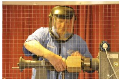
Re-mounting the piece in the chuck jaws using the spigot formed before twisting off, Mark proceeded to clean up the profile and hollowed out the inside by boring the required depth with the spindle gouge (you could use a drill bit to achieve this). Changing to a swan neck gouge the inside was refined and the shoulder cleaned up with a skew gouge.
