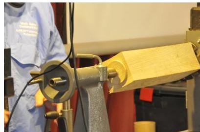
Using a spindle roughing gouge the piece was turned into a cylinder for approximately 70% of its length. Changing to a bowl gouge the shape of the base of the box was made and a shearing cut used to refine the shape. When doing this ensure the flute is in the direction of travel to avoid jams.
