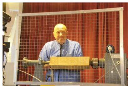
Using a 4 x 4 square ash, which is notorious for 'crazy grain' was mounted using steb centres between centres and a spigot cut on both ends retaining the square edge whilst doing so.
