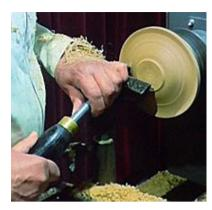
Tom demounted the piece, took off the back plate and mounted it in the chuck jaws to work on the face, firstly taking out the bowl and removing any signs of the screw holes from the faceplate. He formed the "S" shape (ogee) rim and created an inner profile edge, taking lighter and more careful cuts as he did so in order to get the best pre-sanding finish.
