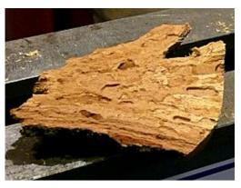
The splits became a little more noticeable so Tom described his method of filling them by putting a wall of Playdoh around the edge to form a retaining "wall" and putting tape on the underside. The split would then be filled with coloured epoxy resin. Copper and bronze powders were mentioned.
