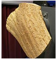
He started the lathe slowly and began cutting the three edges very carefully as most of the time he was "cutting air" and also to avoid breakout on the corners. This helped establish where the upper edge would be.
