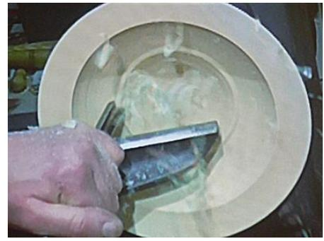
The tool will always follow the angle of the bevel, so by manipulating the tool almost any angle can be achieved - from straight sided to a round side of the bowl. Darren recommends that you practice your cuts on smaller blanks building up your skills and muscle memory. Mass material can be removed quickly with a long grind but the finish will not be as good so practice finishing cuts with a standard 45 degree bowl gouge. Never force a cut always try to stay in control.
