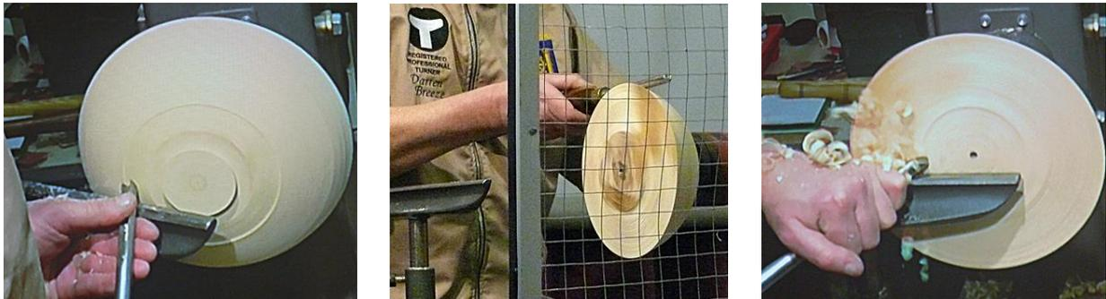
Darren emphasised the importance of having your body weight correctly balanced at all times, pivoting your hips and not moving your feet. Cutting 'uphill' with a standard grind produces a good finish. A reference point was made in the centre of the spigot as the piece was wet wood and bound to distort.
