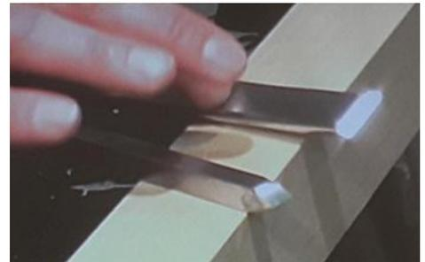
He also used a skew ground at a slight angle and a beading/parting tool which was ground square.
