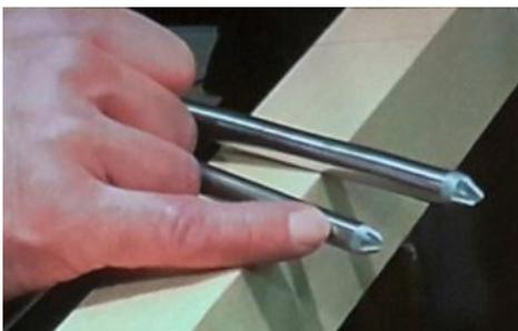
In this demonstration Richard used a spindle gouge with a 35 degree bevel with a secondary bevel on the heel to avoid bruising the wood and giving better access to coves and beads. This was to be the first of four legs which would all have a barley twist finish.
