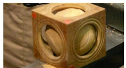
As this picture shows the 'Cup Chucks' were made from a piece of sycamore mounted by a spigot and using a Simon Hope carbide tool the shape and size of the hole was defined. A groove was cut in the front rim of each piece and an o-ring was inserted and secured by super glue. This jig enabled the ball to be held and turned whilst the block was stationary and without marking the sphere.
