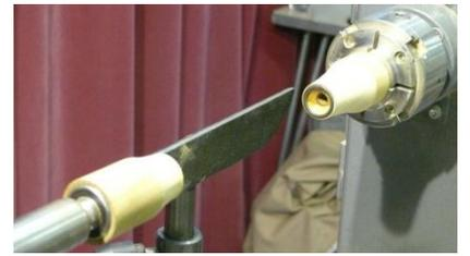
With another jig Paul was able to hold the block securely and free from the sphere to enable final cleaning of the ball with light touches from scrapers.
