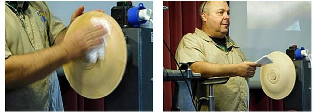
This minimised the airborne dust which could be seen falling to the floor. The sanding pad clogged quickly but was just as quickly cleaned using a small stiff brush.
