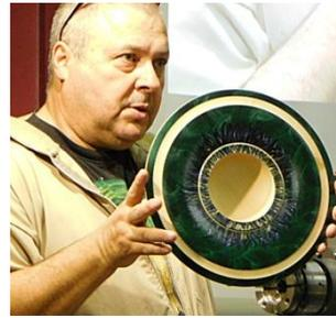
The centre was turned away with Mick explaining how to avoid the "pimple" in the middle by adjusting the angle of approach with the bowl gouge. He even added a micro bevel to his gouge to help make this happen.
