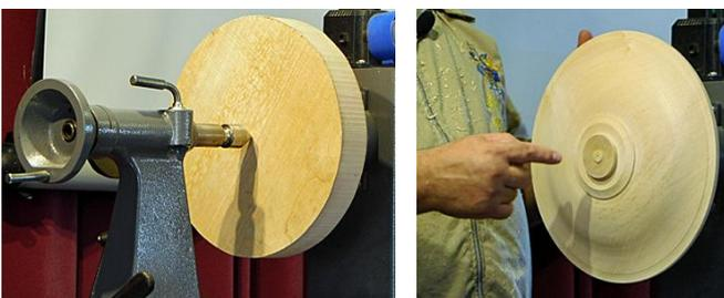
A sharp gouge and good tool control was important to overcome grain tear out but the final finish would be with a 240 grit Rhynogrip abrasive disc and pad mounted on a drill.
