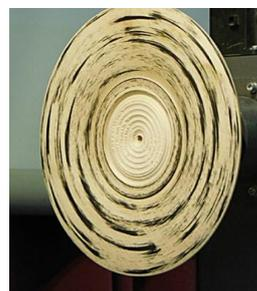
The bowl was turned and mounted on the spigot and Mick formed a curved profile to the outer edge, adding an inner accent groove.
