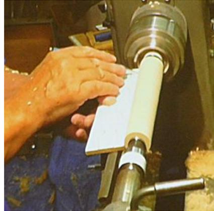
The individual diameters of each stage were then formed by making a groove to the correct diameter with a parting tool. This enabled the initial shape and beads to be formed if confident using a skew or a spindle gouge .
