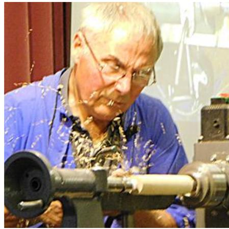
Paul again having marked the blank from the template cut the grooves in key places which determined the diameter before using a beading tool .
