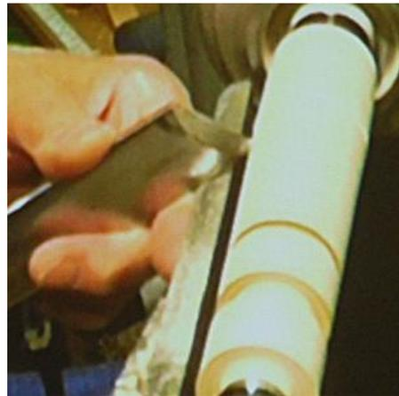
Having successfully turned one leg the end spigot was turned parallel to fit the holes in the seat they must not be tapered. The other 3 legs followed the same procedure.
